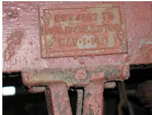
Figure 12: Before treatment detail of the cover of one of the journal boxes.
