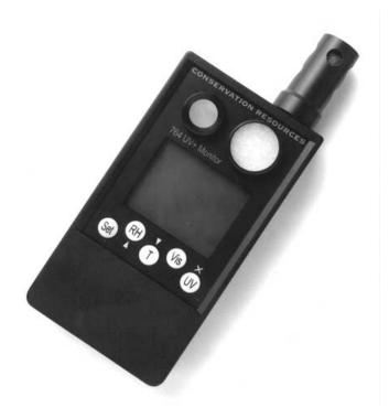
The light meter in the kit has been upgraded to the ELSEC model 764. This meter measures both visible and ultraviolet (UV) light that formerly were measured using two instruments in this kit. Both visible and ultraviolet light readings should be recorded and kept on file for future reference on a form such as the sample on page 9.
