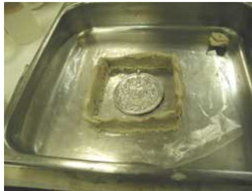
Figure 2: A dam of Klean Klay modeling clay is built around the Medal to contain the molding compound.
