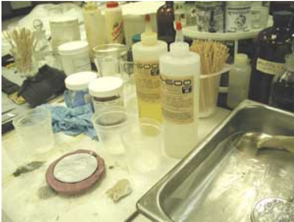
Figure 5: General view of the molding and casting supplies. The polyurethane 2-part casting compound is in the two containers in the center.
