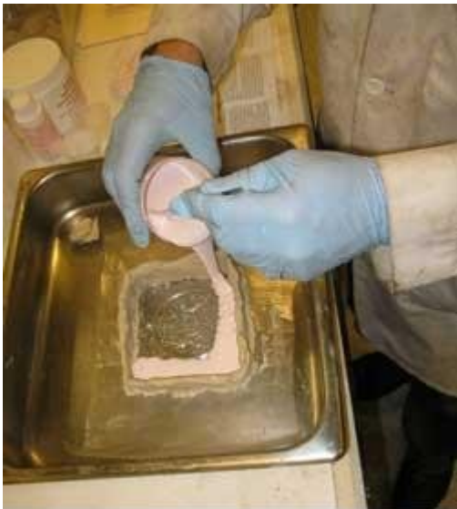
Figure 3: The two components of the silicone RTV mold compound are mixed in a disposable plastic beaker prior to pouring the compound over the Medal.
