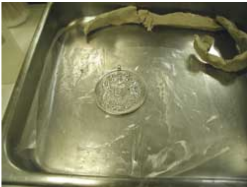
Figure 1: The peace medal is set in a steel pan on silicone release film.
